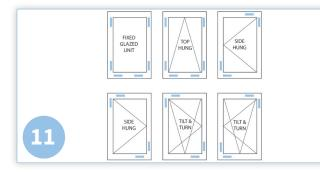
Ensure that you follow these guidelines for 'toe and heeling' the glass otherwise you could have operational issues when opening and closing any sashes. If you find the sash is catching at the bottom when used you will need to insert more glass packers in the top corner of the handle side, this will push the sash up.
