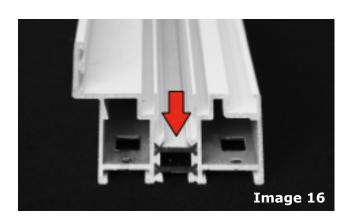
You can fix the frame through the polyamide thermal break as indicated on image 16, we advise you to pilot drill first to ensure that it does not crack, care should be taken not to over-tighten the fixings which should not break through the thermal barrier.
